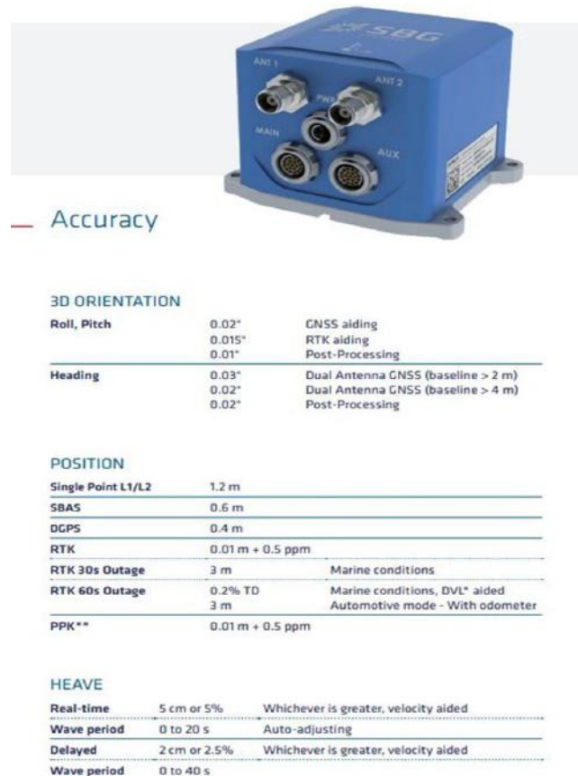
Figure 5: SBG Equinox (IMU) Technical Specifications
